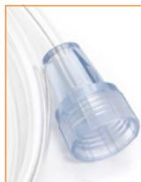
Available with oxygen tubing featuring a universal connector, which can be attached to a 6mm flow meter spigot or fitted directly onto a 9/16-18 UNF Diameter Index Safety System (D.I.S.S.) flow meter
