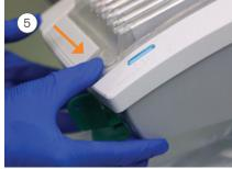
Push the cassette down and and the latch forward, ensure location by checking that the latch is flush with the front of the InterCooler<sup>™</sup> housing (see fig.1 below)
