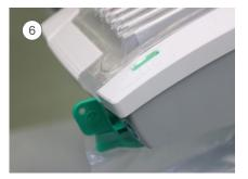
The button will illuminate green if the system is set up and functioning correctly
